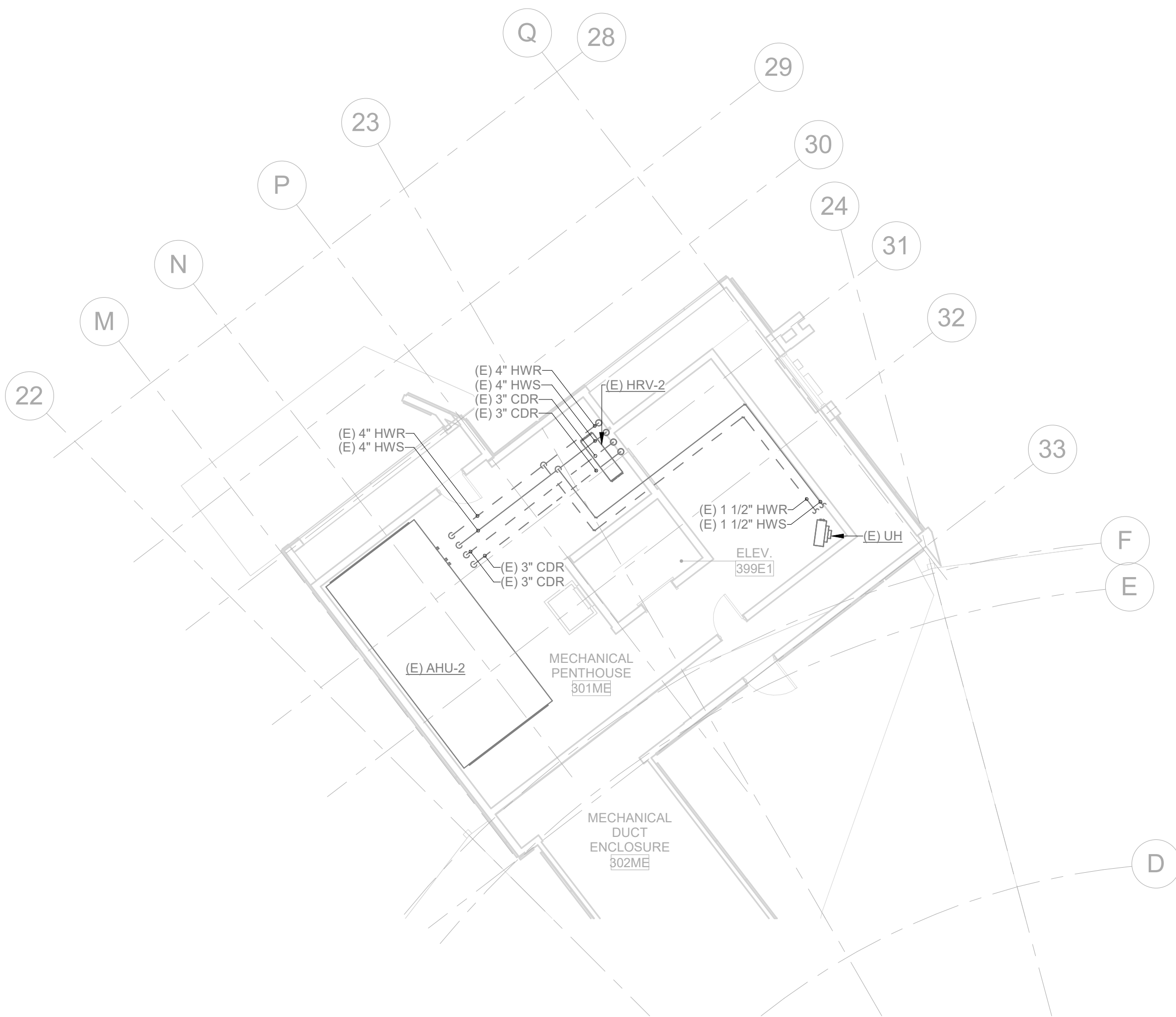
2 MECHANICAL PENTHOUSE - MECHANICAL PIPING DEMO PLAN N.T.S.
