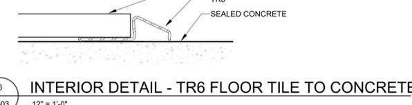
6 INTERIOR DETAIL - TR6 FLOOR TILE TO CONCRETE
