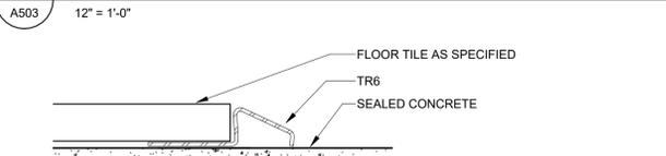
6 INTERIOR DETAIL - TR6 FLOOR TILE TO CONCRETE
