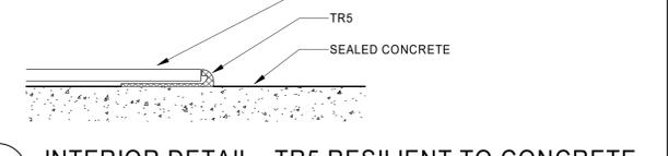
5 INTERIOR DETAIL - TR5 RESILIENT TO CONCRETE
