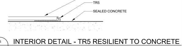
5 INTERIOR DETAIL - TR5 RESILIENT TO CONCRETE
