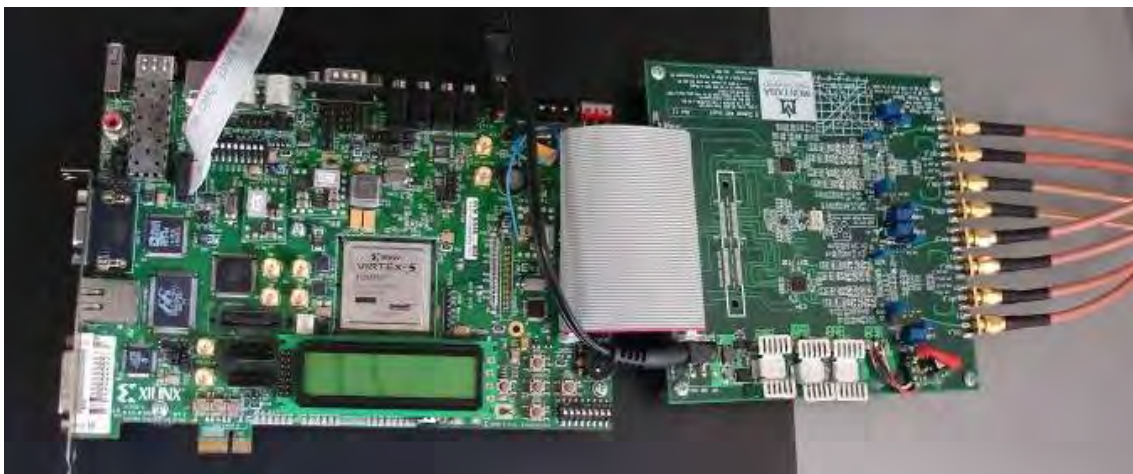
Figure 3.5 Xilinx ML507 board containing the Virtex-5 FX70 FPGA connected to a custom 8-channel ADC board.
