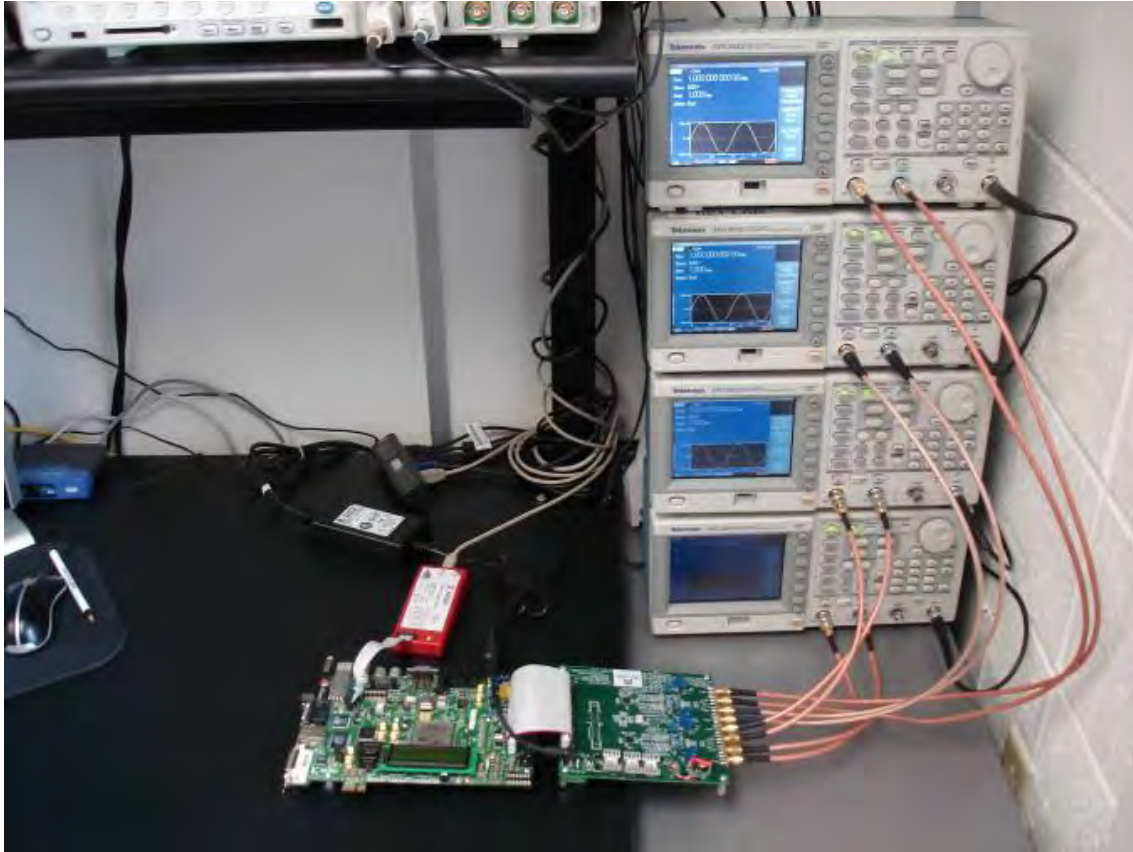
Figure 3.9 Testbed for the DOA estimation verification. The signal generators emulate 8 down converted carrier signals with phases corresponding to an arbitrary incident angle as observed by the 5.8GHz circular antenna array.
