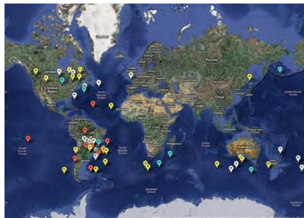
Figure 17: Location of SEEs during GSFC SpaceCube Deployment (Virtex-4) on MISSE-7 over 10 month Period [31].
